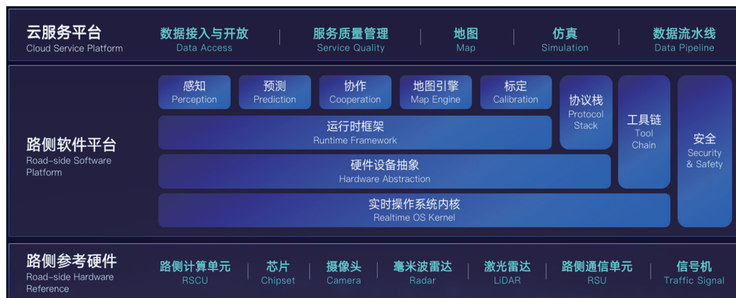
Figure 6.2 Overall Architecture of Vehicle-infrastructure Collaboration Open Platform 2.0
